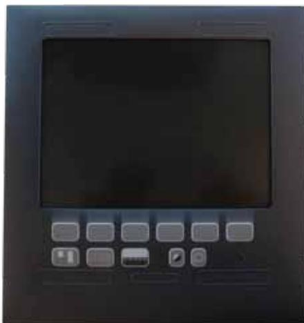
**The SA-C112 is a Sub assembly frontplate with LCD for the SKIPPER DL850 270 kHz Navigational Doppler Speed Log.**
